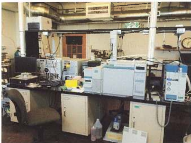
Volatiles: Agilent 8260 GC/MS w computer (16' bench) With purge and trap on right. GCMS will be replaced; Purge and trap will be used in new facility.
