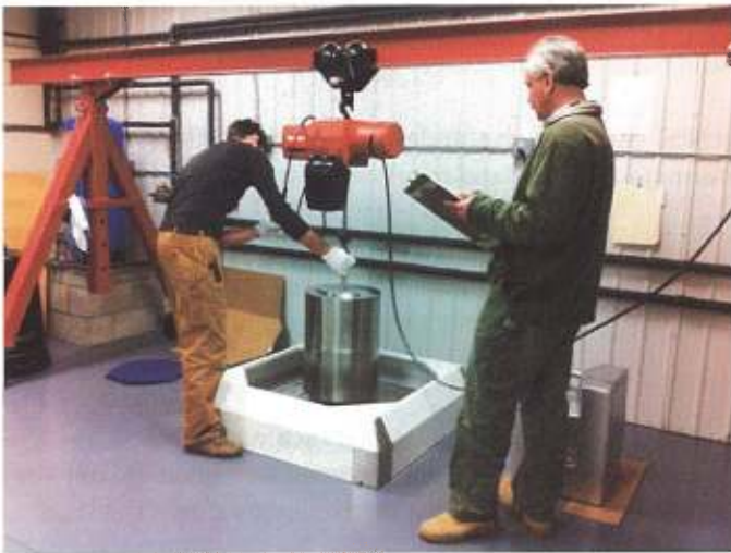
Gantry beam lifting a proving mass (or standard).
