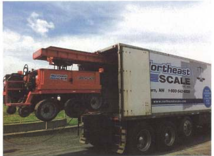
Weight cart arriving with its own unloading beam.
