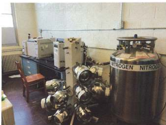
Volatiles, left to right: TO-15 GCMS, 7100 concentrator (will get 7200), canister tree, nitrogen dewar
