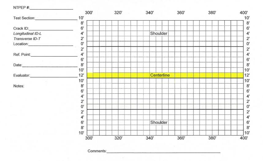
Table 7: Crack Sealant Field Evaluation Worksheet - 400'-500' Test Sub-Section
