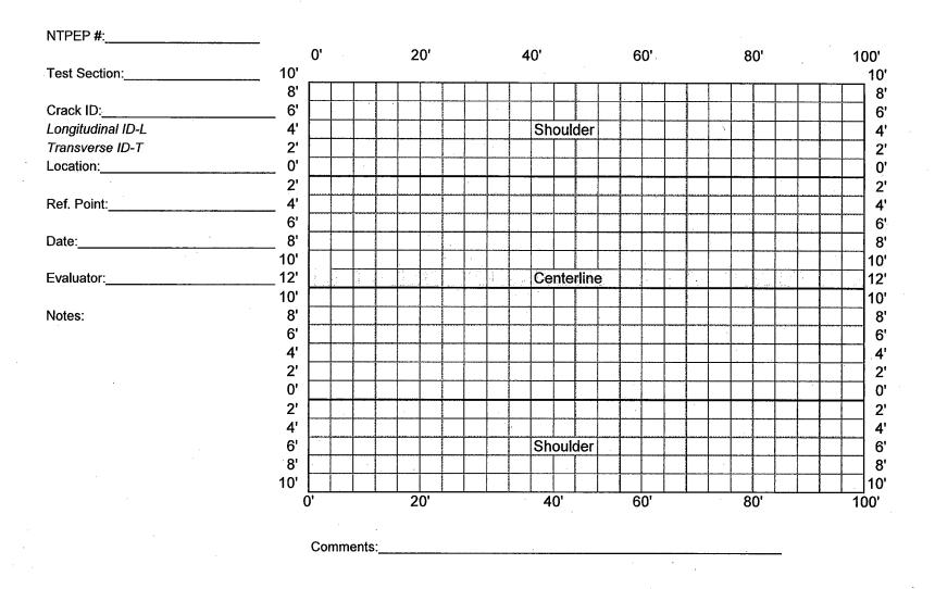
Table 3: Crack Sealant Field Evaluation Worksheet - 0-100' Test Sub-Section
